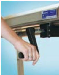
Quickly, easily adjust table surface to heights between 30" and 42"
